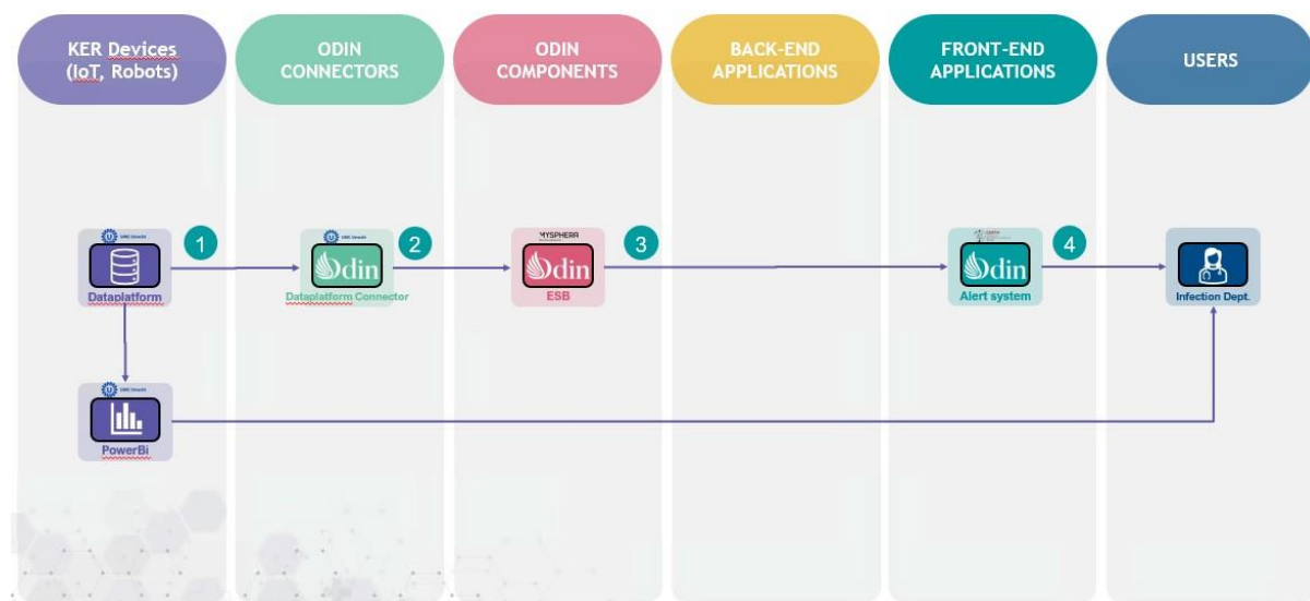
Figure 35. UMCU UML diagram of the data visualization process and alert system when the concentration of a certain pathogen is above threshold.
